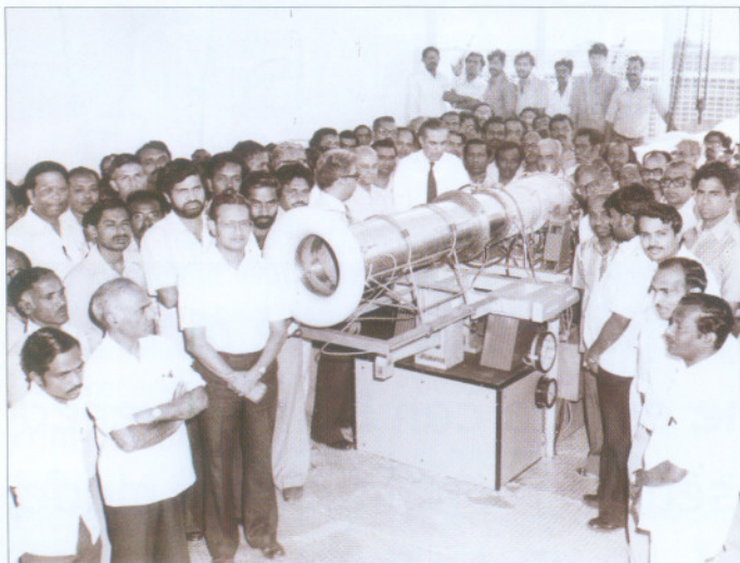
Proving of flame tube of PTAE in Test Bed
