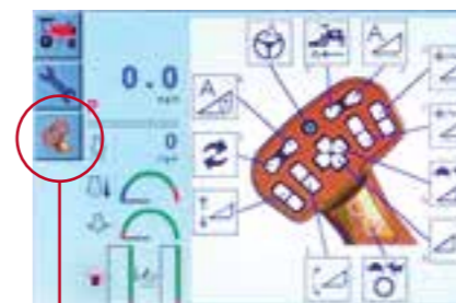
A handle configuration icon in the FieldMax Monitor will always be visible, so you can view and/or change handle settings with a single button.
