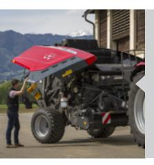
Full width side doors provide easy access for maintenance. The smooth surface design prevents dust accumulation beneath the panels while secure locking prevents unintended opening and potential damage.
