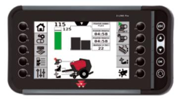
The **E-Link Pro** monitor with integrated ISOBUS technology features a large bright screen which offers great visibility of multiple parameters, giving the operator more information and control of the baler.
