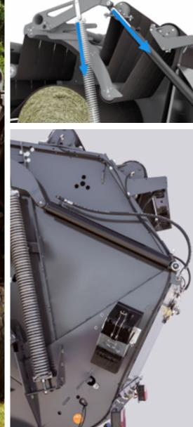
Bale volume increases exponentially in relation to its diameter, together with a corresponding belt pressure, to keep the bale density constant.
