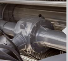
The Powersplit gearbox equally divides and transfers power to drive the rotor unit on one side and the roller drives on the other, reducing the overall power requirements by simplifying the drivelines. This results in a more efficient baler which uses less fuel.
