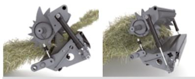
In the event of a blockage the operator can easily open the feed table floor and lower the knives at the same time to provide enough space for material to pass through.
