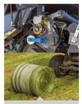
The optional Variotwin twine system offers simple and economical bale tying. The unique Variable Speed Control allows for additional twine revolutions on the bale edges, securing bale ends and increasing overall tying speed, which is particularly beneficial when baling light crops.
