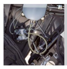
Automatic chain lubrication with individual adjustment for each chain guarantees sufficient oil supply, reduces maintenance time and extends chain service life. For added durability the highest quality chains are used throughout the baler.
