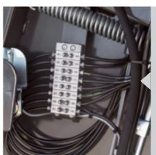
Regular and sufficient lubrication of roller bearings is extremely important, particularly in adverse conditions, for example when baling silage. Centralized grease banks for roller bearing lubrication are located in convenient positions for easier access and reduced service time.
