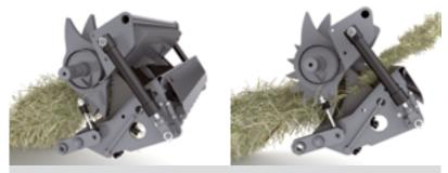
The patented protection system prevents peak loads from turning into blockages by gentle lowering of the floor which is suspended on rubber blocks or steel springs, depending on the model.
