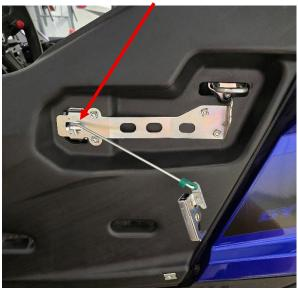
10.Reinstall the handle latch using the two 10mm bolts that were removed in step 2. "Be sure you align the latch as accurately as possible with the latch ring so that your door will close and open nicely."
