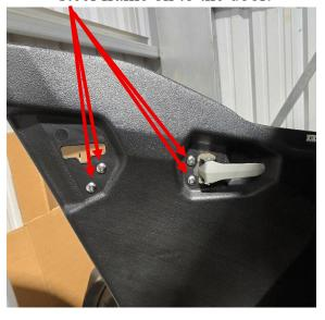
4. Remove the stamped steel frame and door handle from the door frame.
