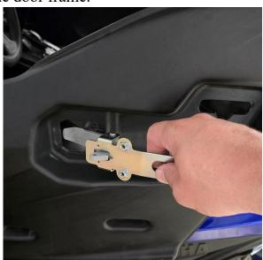
5. Remove the c-clip and pull the pin to remove the factory handle from the steel frame. Wipe
