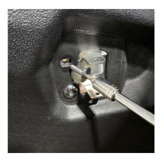
7. Install the new billet handle! "You may need to squeeze or slightly spread the two steel ears so that they align in the slots on the new handle."
