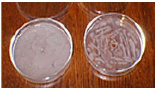
Dr James Harkryder, Cypress College Biology Dept. Test of biostimulants in Launch. Heterotrophic plate count, left petri with 2 drops of 100% bio-stimulant, right petri 2 drops of 10% diluted bio-stimulant.
