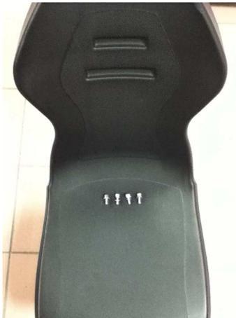
Step3: Remove 2 airbag screws.
