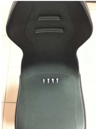
Step3: Remove 2 airbag screws.
