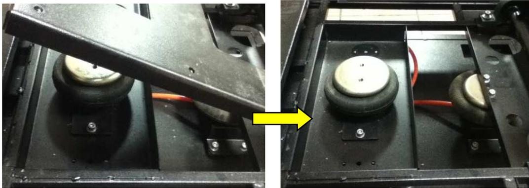
Step5: Remove 2 fixation screws.
