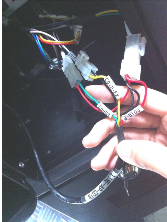
1. **“Coin-P”** input power 12V to the coin acceptor.
