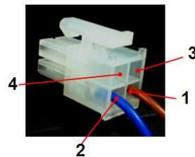
2. **“Coin-Ex”** output credit signal from the coin acceptor
