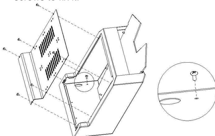
**Step6:** Connect the power cable inside the light set and use Screw to fix the cover.
