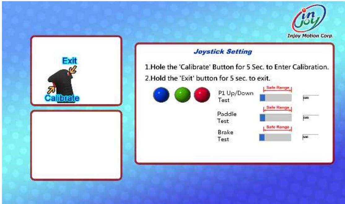
To calibrate the Pedal and Brake, follow the directions on the screen and go through these steps.
