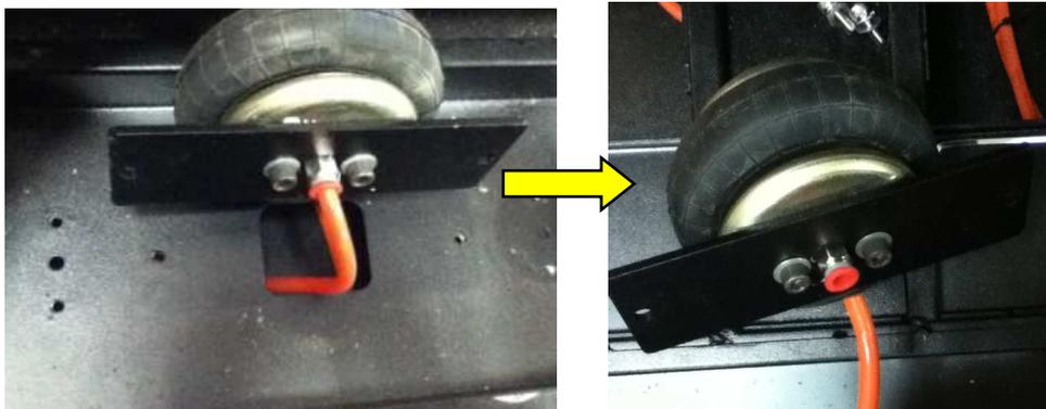
Step7: After changing, lock 2 airbag screws, tube, and 2 fixation screws.
