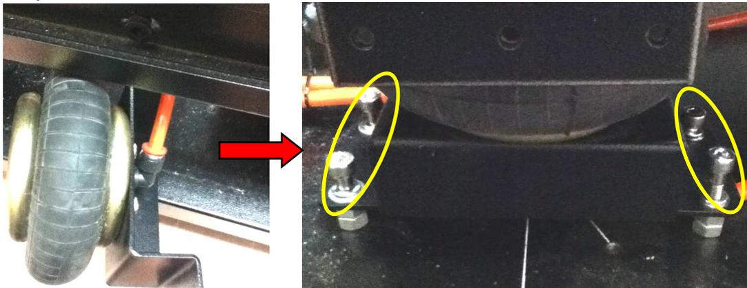
Step9: Install 2 airbag screws. <Finish>
