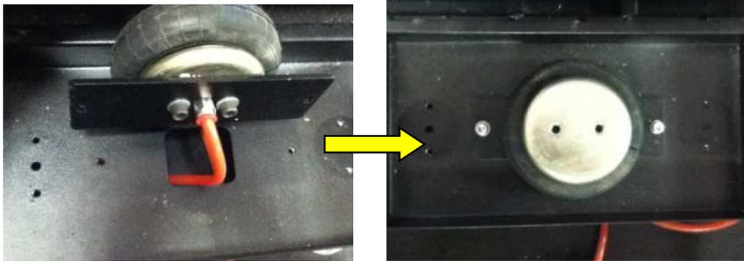
Step8: Cover the seat base, tighten 2 airbag screws.
