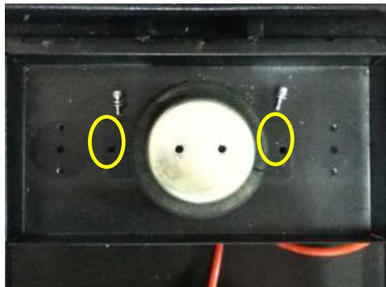
Step6: Remove the tube and screws, and change airbag.
