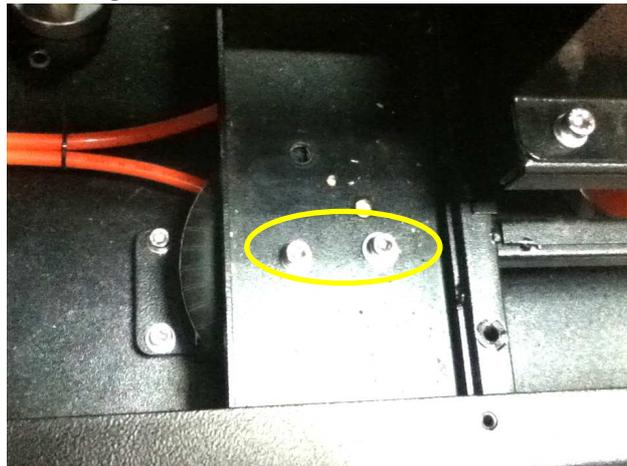
Step3: Remove 4 fixation screws.
