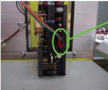
This pin is for coin mechanism
