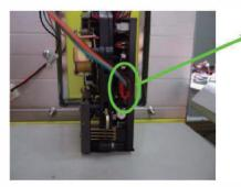
This pin is for coin mechanism
