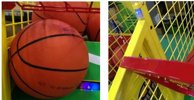
**Ball gate is inverted (gate closes when credited):** Check that J17 and the connector near power supplier is connected well. If it still malfunctions, test the proximity sensor.
