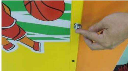
8. Attach the L shape bracket onto the back of the console box. Use the larger screws to mount the L shaped bracket.
