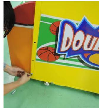
5. Unscrew both screws a little bit in order to remove the console unit easier.
