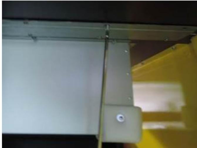
3. Fit a screw, spring washer, & flat washer to mount the metal bracket of Right and Left Metal Net
