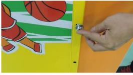
8. Attach the L shape bracket onto the back of the console box. Use the larger screws to mount the L shaped bracket.
