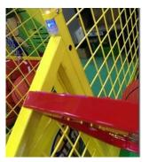
**Ball gate is inverted (gate closes when credited):** Check that J17 and the connecter near power supplier is connected well. If it still malfunctions, test the proximity sensor.
