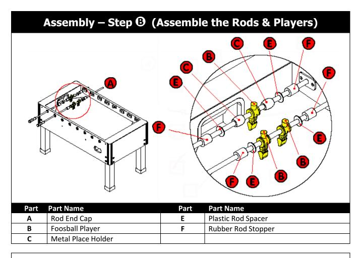
\*IMPORTANT NOTE\* We recommend assembling all the pieces on the playfield first (*before tightly securing the players to the rods*) to make sure all the players are in the right position. Continue to STEP ③ to tightly secure the players once you're positive everything is placed according to the aerial view.
