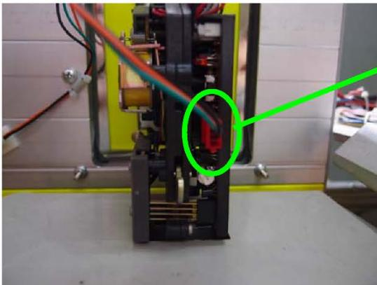
This pin is for coin mechanism
