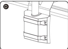
Tighten the Plastic Bar Bracket covers completely once both are attached.
