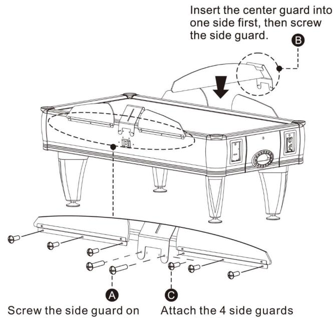
Screw the side guard on one side with flathead screw M5x15mm(4)
