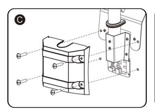
Insert the Plastic Bar Bracket Cover into the notch of the Rubber Cover and attach it with the M5X35 screws.
