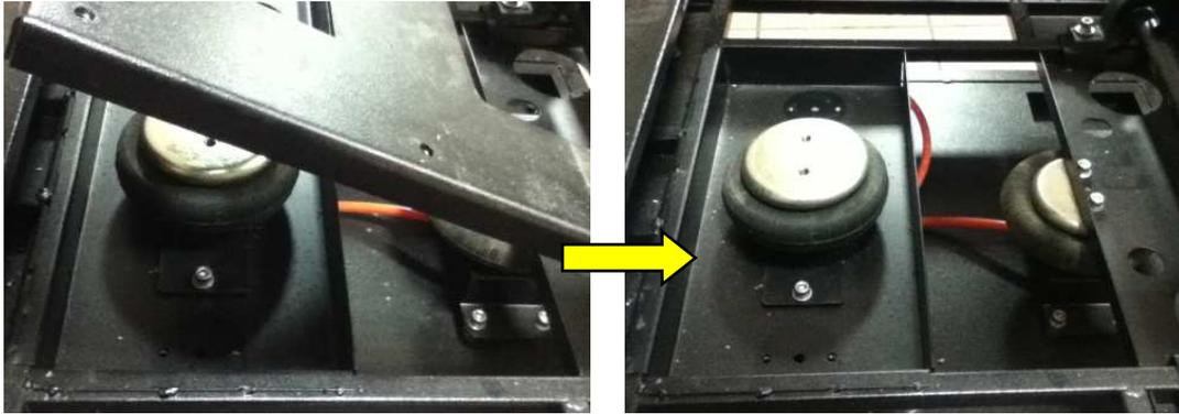
Step5: Remove 2 fixation screws.
