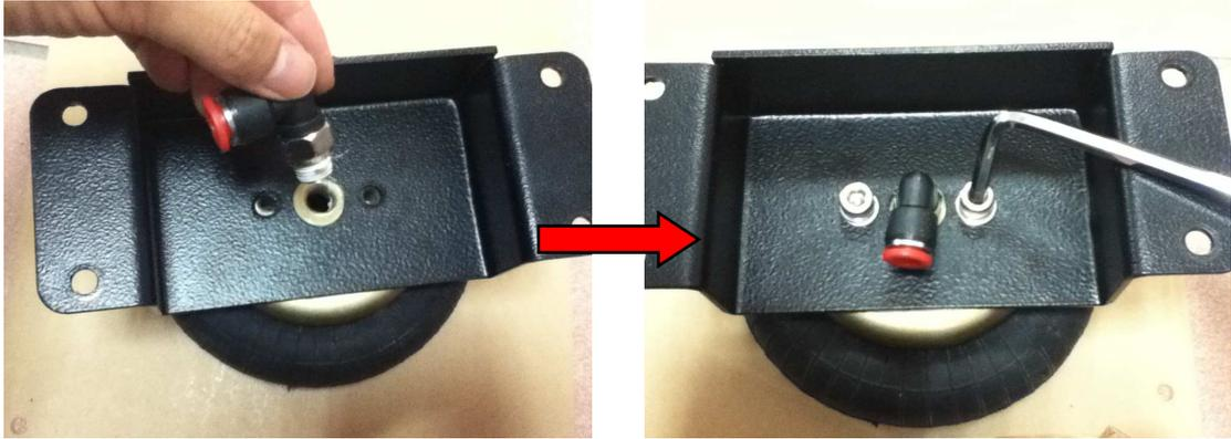
Step8: Install 4 fixation screws.
