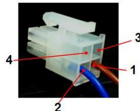
2. **“Coin-Ex”** output credit signal from the coin acceptor
