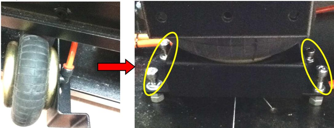
Step9: Install 2 airbag screws. <Finish>
