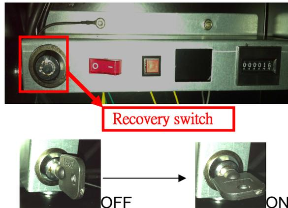
**Step1:** When the screen shows “insert coin”, Use the key specified for recovery switch and turn it right.
