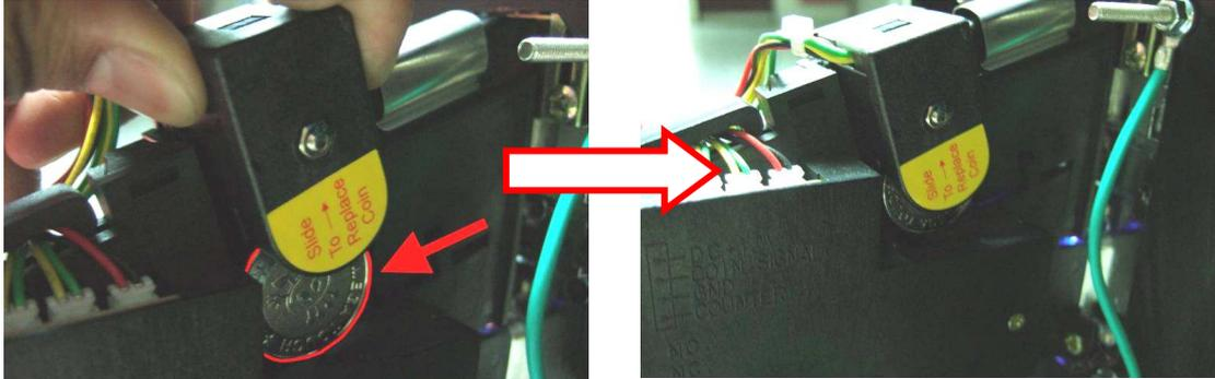
**Step9:** Check the Coin Acceptor Setting. (Select “NO” on top switch, “SLOW” on bottom switch)
