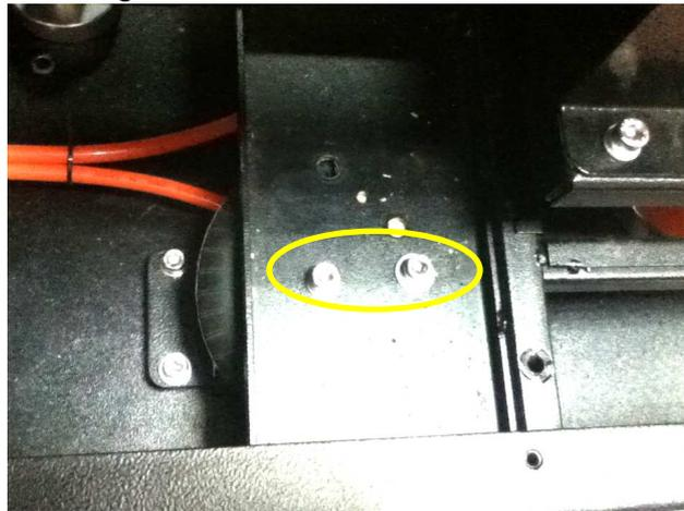
Step3: Remove 4 fixation screws.
