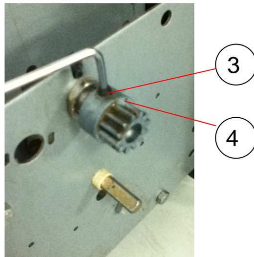
Step6: Install gear②, and make sure gear④ close to second tooth of the gear②.
