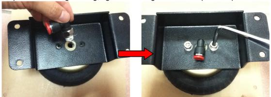
Step8: Install 4 fixation screws.
