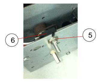
Step3: Use meter to measure resistance value between pin2 and pin3 of the potentiometer, and make sure 1.6Kohm for pedal, 2.6Kohm for brake.
