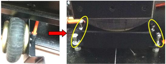
Step9: Install 2 airbag screws. <Finish>
