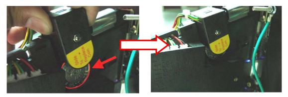
Step9: Check the Coin Acceptor Setting. (Select "NO" on top switch, "SLOW" on bottom switch)
