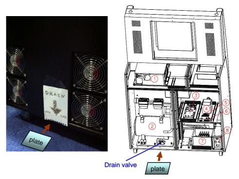
Note: The air compressor tank drains water after machine power off. So it is necessary to put a container on the floor and right under the drain valve to catch the water. Generally, a plastic plate around 25x20x3(LxWxH)cm is suggested.
