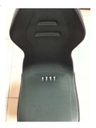
Step3: Remove 2 airbag screws.
