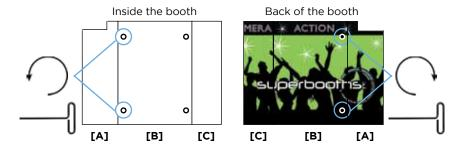
7. Align the middle wall [B] with the back wall [C]. Use the included hex key to lock the wall together.
