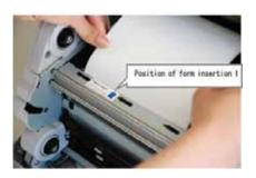
5. Fit the paper to the proper position for each size. L and 2L paper (6") correspond to the L line.
