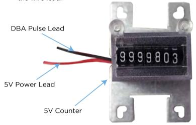
2. Use the screws included to mount the 5V Counter to the side wall of the 40" Monitor inclosure.
