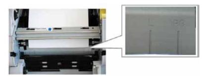
6. The black form is inserted under the form guide. Insert the paper in the direction of the arrow until you hear a beep (close to the line shown below). When doing this, insert the paper straight. If it is not inserted straight it could cause white lines on the print, ribbon wrinkles, and register slippage.
