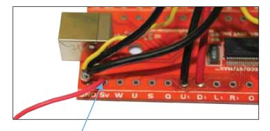
Red wire lead connects to 5V on the credit board.
