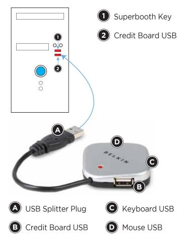
2. Plug in the USB Splitter to the now open USB port. Now plug in the Credit Board into the first USB slot, the keyboard in to the second USB slot, and the mouse into the third USB slot. Restart the PC.
