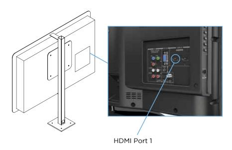
8. Chase the HDMI cable and the monitor power cord through the chase hole on back of the topper mount.
