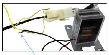
Solder the twisted wires to ensure a proper connection.
