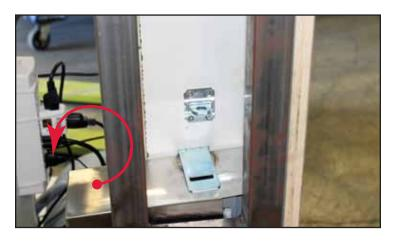
4. To replace the Lock Box lift it up and set it on the DBA. Lift the hasp onto the staple and place your lock back on the staple.
