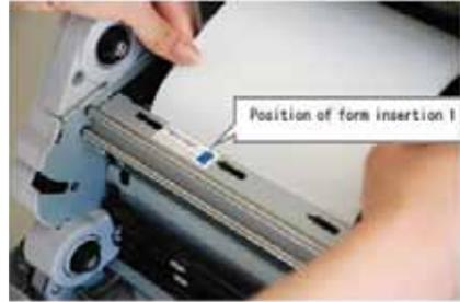
5. Fit the paper to the proper position for each size. L and 2L paper (6") correspond to the L line.
