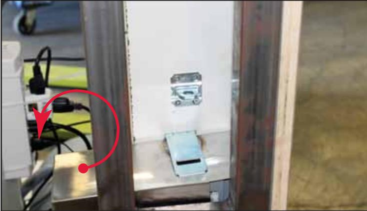
4. To replace the Lock Box lift it up and set it on the DBA. Lift the hasp onto the staple and place your lock back on the staple.
