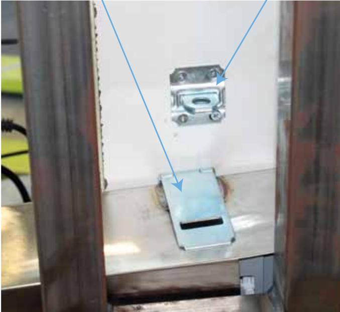
6. To mount your lock box to secure the DBA slide the metal box over the DBA and slide the hasp over the staple. Use you own lock to slide it through the staple to secure the DBA.
