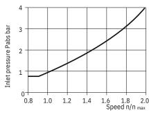
Note: max. permissible speed nmax perm.(speed limit) min. permissible inlet pressure at port S admissible values for the drive shaft seal
