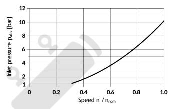
This diagram is valid only for the optimum viscosity range from  $v_{opt} = 36 \text{ to } 16 \text{ mm}^2/\text{s}.$
