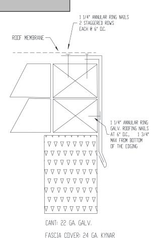
SE SERIES EDGINGS ARE AVAILABLE IN VARIOUS METALS. THEY ARE ES-1 TESTED IN 24 GA. STEEL AND .040 ALUMINUM. MAXIMUM TESTED FACE SIZE IS 8". CALL ULTRA SEAM FOR DETAILS.
