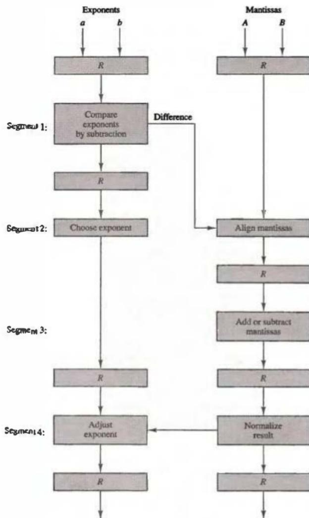
Figure 9-6 Pipeline for floating-point addition and subtraction.
