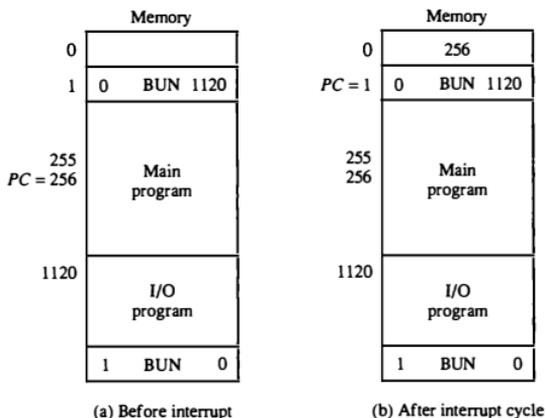
read from memory during the fetch phase, control goes to the indirect phase (because  $I = 1$ ) to read the effective address. The effective address is in location 0 and is the return address that was stored there during the previous interrupt cycle. The execution of the indirect BUN instruction results in placing into PC the return address from location 0.
