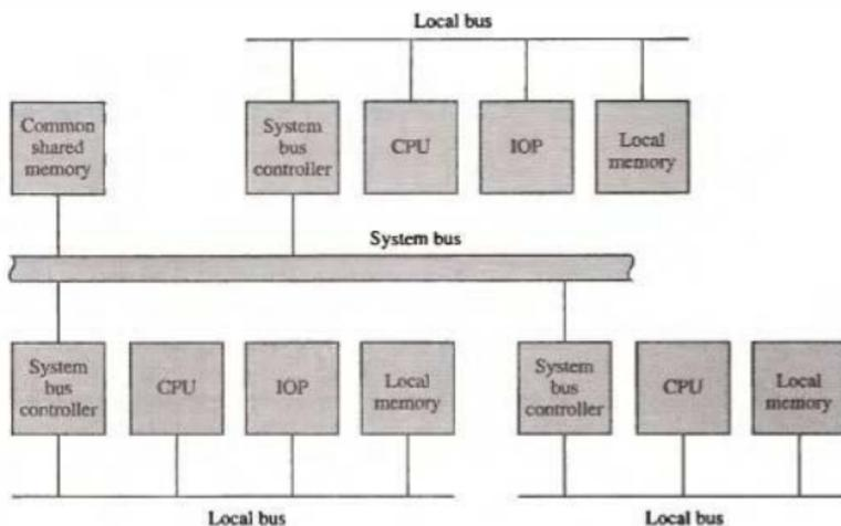
Figure 13-2 System bus structure for multiprocessors.
