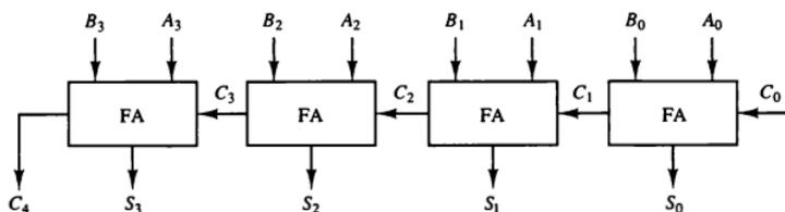
Figure 4-6 4-bit binary adder.
