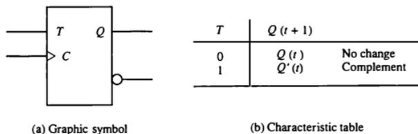
Figure 1-22 T flip-flop.
