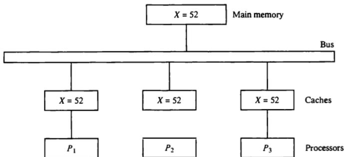
Figure 13-12 Cache configuration after a load on  $X$ .
