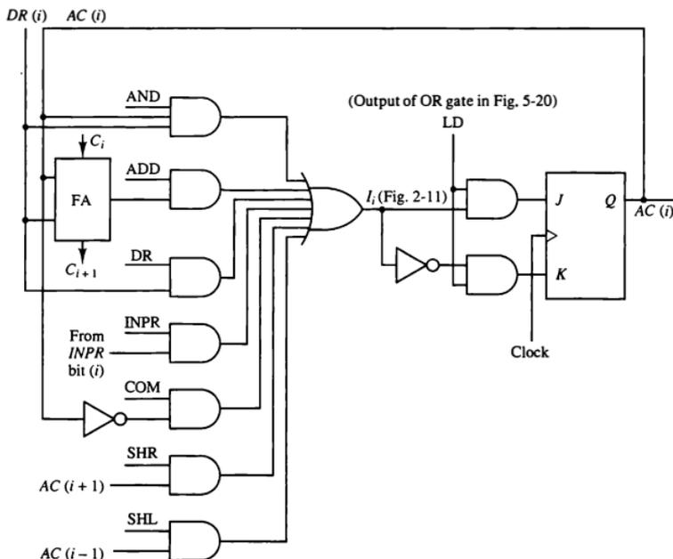
full-adder with the corresponding input and output carries. The transfer from *INPR* to *AC* is only for bits 0 through 7. The complement microoperation is obtained by inverting the bit value in *AC*. The shift-right operation transfers the bit from  $AC(i + 1)$ , and the shift-left operation transfers the bit from  $AC(i - 1)$ . The complete adder and logic circuit consists of 16 stages connected together.
