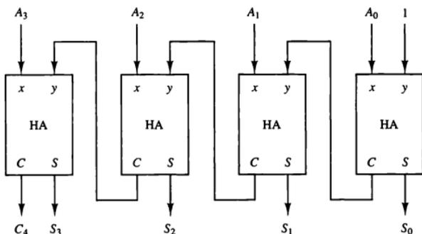
Figure 4-8 4-bit binary incrementer.
