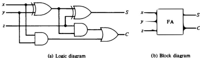
Figure 1-18 Full-adder circuit.
