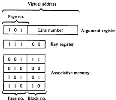
block number. The page field in each word is compared with the page number in the virtual address. If a match occurs, the word is read from memory and its corresponding block number is extracted.
