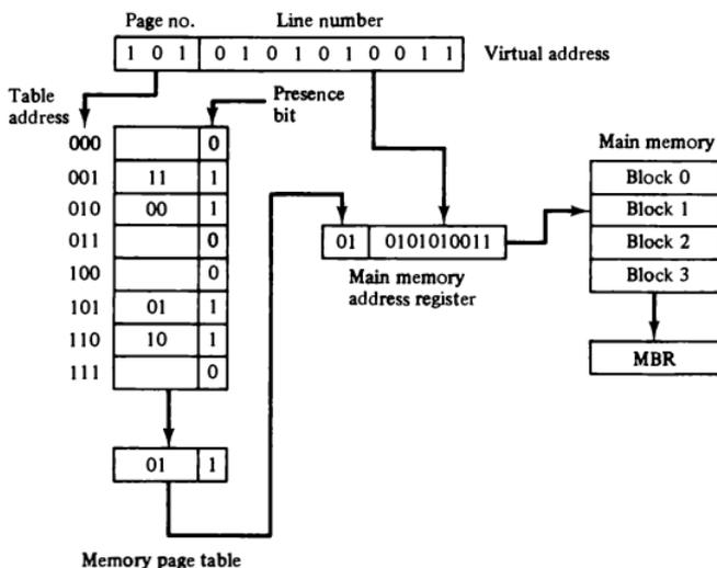
transfers the content of the word to the main memory buffer register ready to be used by the CPU. If the presence bit in the word read from the page table is 0, it signifies that the content of the word referenced by the virtual address does not reside in main memory. A call to the operating system is then generated to fetch the required page from auxiliary memory and place it into main memory before resuming computation.
