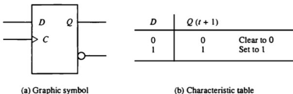
Figure 1-20  $D$  flip-flop.
