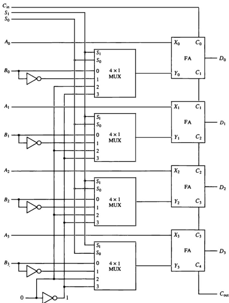
Figure 4-9 4-bit arithmetic circuit.
