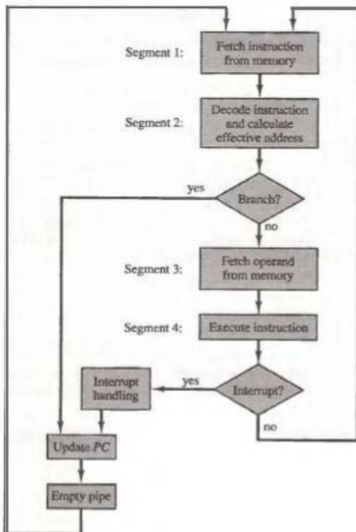
Figure 9-7 Four-segment CPU pipeline.
