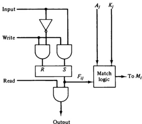
We now include the key bit  $K_j$  in the comparison logic. The requirement is that if  $K_j = 0$ , the corresponding bits of  $A_j$  and  $F_j$  need no comparison. Only when  $K_j = 1$  must they be compared. This requirement is achieved by OR'ing each term with  $K_j'$ , thus:
