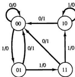
Figure 1-26 State diagrams of sequential circuit.
