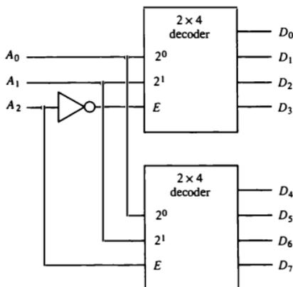
The example demonstrates the usefulness of the enable input in decoders or any other combinational logic component. Enable inputs are a convenient feature for interconnecting two or more circuits for the purpose of expanding the digital component into a similar function but with more inputs and outputs.
