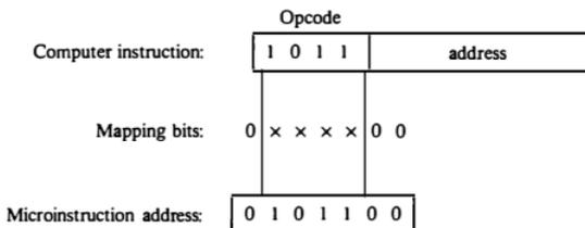
The mapping function is sometimes implemented by means of an integrated circuit called programmable logic device or PLD. A PLD is similar to ROM in concept except that it uses AND and OR gates with internal electronic fuses. The interconnection between inputs, AND gates, OR gates, and outputs can be programmed as in ROM. A mapping function that can be expressed in terms of Boolean expressions can be implemented conveniently with a PLD.
