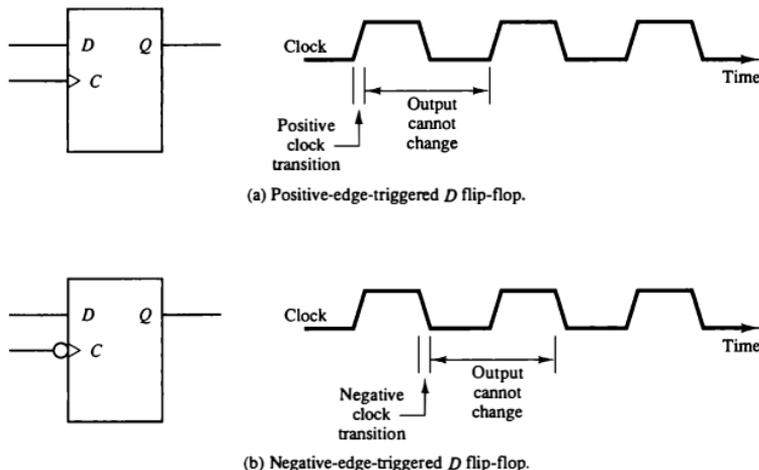
Figure 1-23 Edge-triggered flip-flop.
