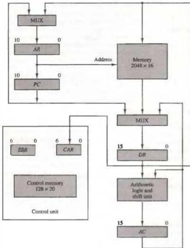
Figure 7-4 Computer hardware configuration.
