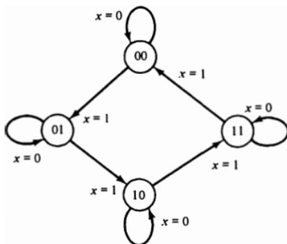
Figure 1-27 State diagram for binary counter.
