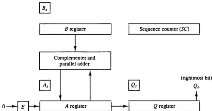
least significant bit of  $A$  is shifted into the most significant position of  $Q$ , the bit from  $E$  is shifted into the most significant position of  $A$ , and 0 is shifted into  $E$ . After the shift, one bit of the partial product is shifted into  $Q$ , pushing the multiplier bits one position to the right. In this manner, the rightmost flip-flop in register  $Q$ , designated by  $Q_n$ , will hold the bit of the multiplier, which must be inspected next.
