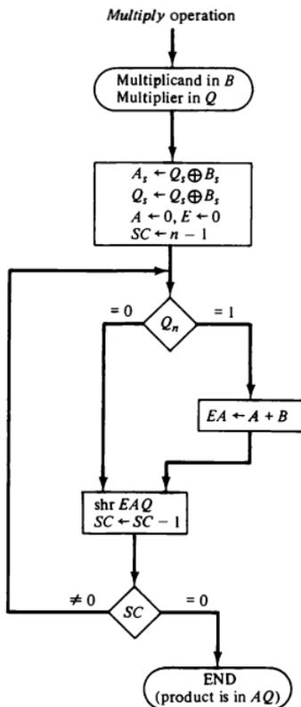
correspond to the sign of the product since a double-length product will be stored in registers *A* and *Q*. Registers *A* and *E* are cleared and the sequence counter *SC* is set to a number equal to the number of bits of the multiplier. We are assuming here that operands are transferred to registers from a memory unit that has words of *n* bits. Since an operand must be stored with its sign, one bit of the word will be occupied by the sign and the magnitude will consist of  $n - 1$  bits.
