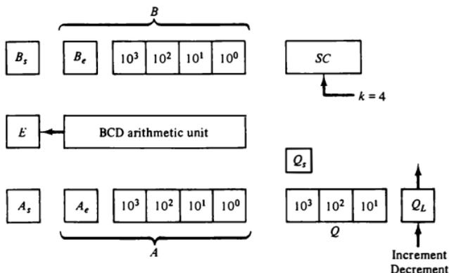
Figure 10-21 Registers for decimal arithmetic multiplication and division.
