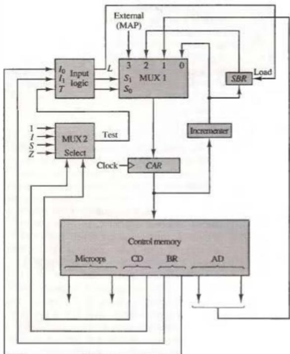
Figure 7-8 Microprogram sequencer for a control memory.
