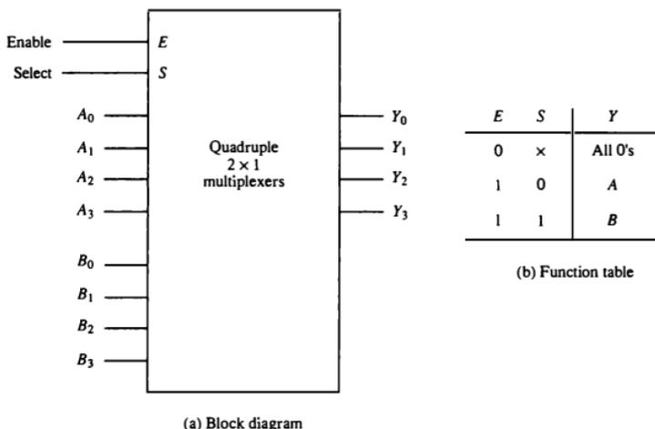
Figure 2-5 Quaduple 2-to-1 line multiplexers.
