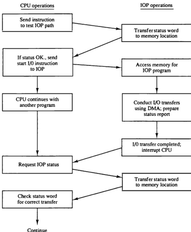
responds by inserting a status word in memory for the CPU to check. The bits of the status word indicate the condition of the IOP and I/O device, such as IOP overload condition, device busy with another transfer, or device ready for I/O transfer. The CPU refers to the status word in memory to decide what to do next. If all is in order, the CPU sends the instruction to start I/O transfer. The memory address received with this instruction tells the IOP where to find its program.
