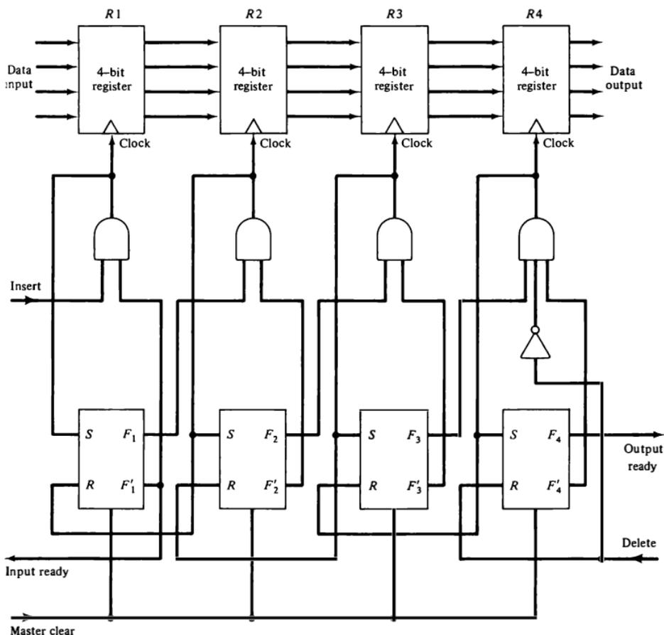
Figure 11-9 Circuit diagram of  $4 \times 4$  FIFO buffer.
