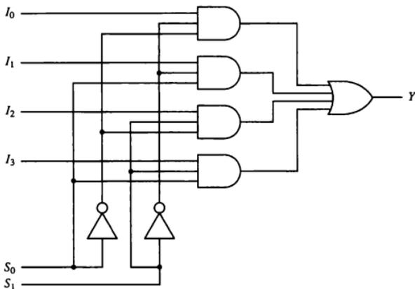
When the selection inputs are equal to 00, output  $Y$  is equal to input  $I_0$ . When the selection inputs are equal to 01, input  $I_1$  has a path to output  $Y$ , and similarly for the other two combinations. The multiplexer is also called a *data selector*, since it selects one of many data inputs and steers the binary information to the output.
