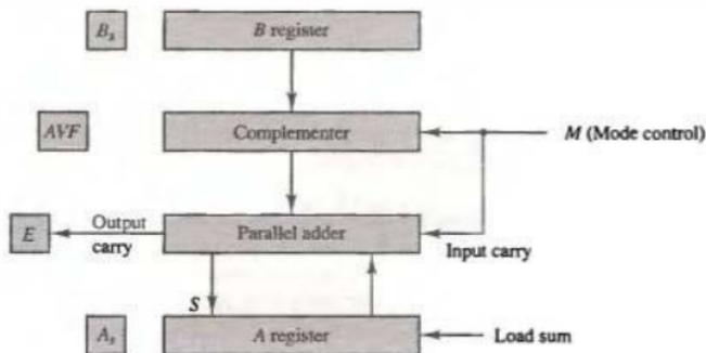
Figure 10-1 Hardware for signed-magnitude addition and subtraction.
