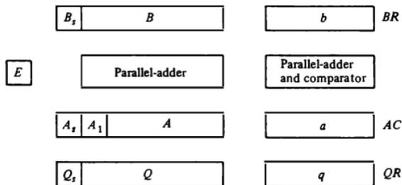
whose sign is in  $A$ , and a magnitude that is in  $A$ . The exponent is in the part of the register denoted by the lowercase letter symbol  $a$ . The diagram shows explicitly the most significant bit of  $A$ , labeled by  $A_1$ . The bit in this position must be a 1 for the number to be normalized. Note that the symbol  $AC$  represents the entire register, that is, the concatenation of  $A_s$ ,  $A$ , and  $a$ .
