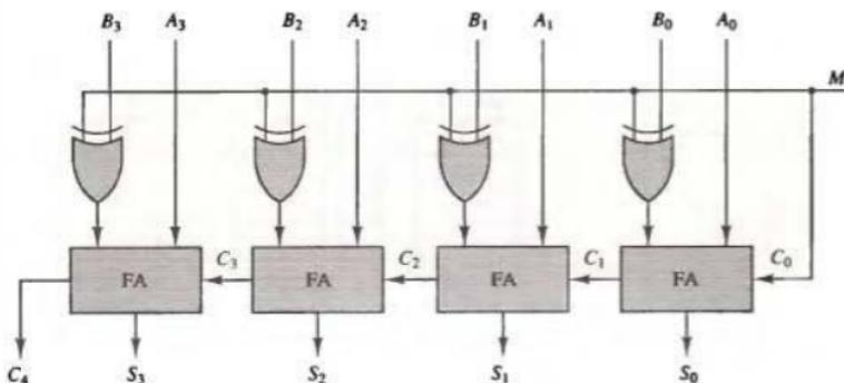
Figure 4-7 4-bit adder-subtractor.
