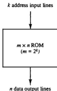
Figure 2-13 Block diagram of read only memory (ROM).
