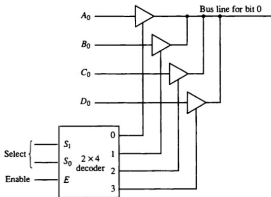
Figure 4-5 Bus line with three state-buffers.
