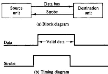
Figure 11-4 Destination-initiated strobe for data transfer.
