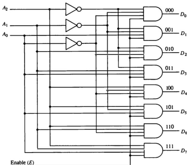
Figure 2-1 3-to-8-line decoder.
