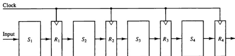
Figure 9-3 Four-segment pipeline.
