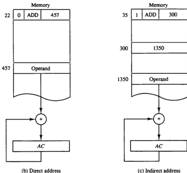
Figure 5-2 Demonstration of direct and indirect address.
