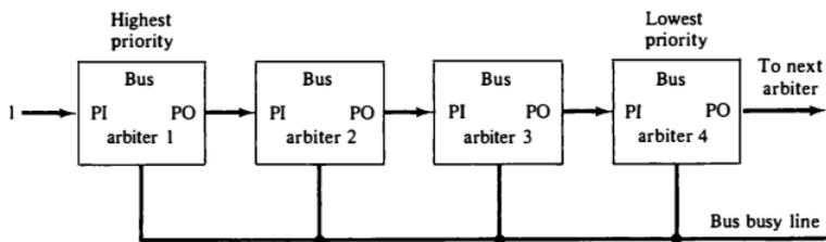
Figure 13-10 Serial (daisy-chain) arbitration.
