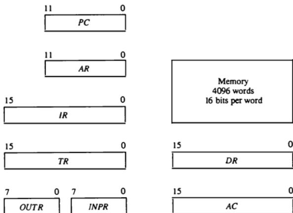
Figure 5-3 Basic computer registers and memory.
