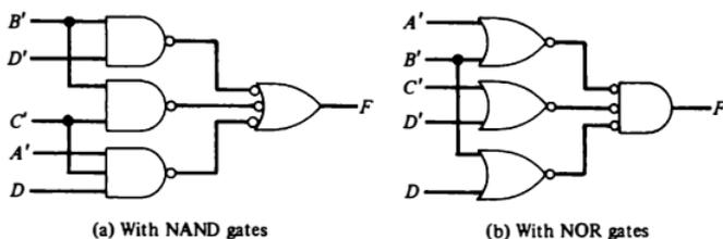
Figure 1-13 Logic diagrams with NAND or NOR gates.
