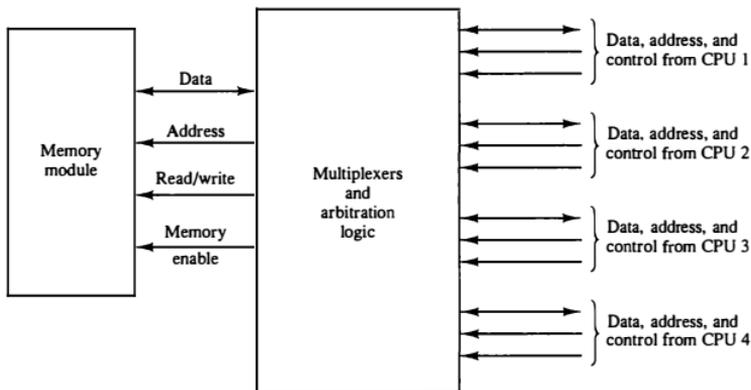
address, and control from one CPU for communication with the memc module. Priority levels are established by the arbitration logic to select one CI when two or more CPUs attempt to access the same memory. The multiplexers are controlled with the binary code that is generated by a priority encoder within the arbitration logic.
