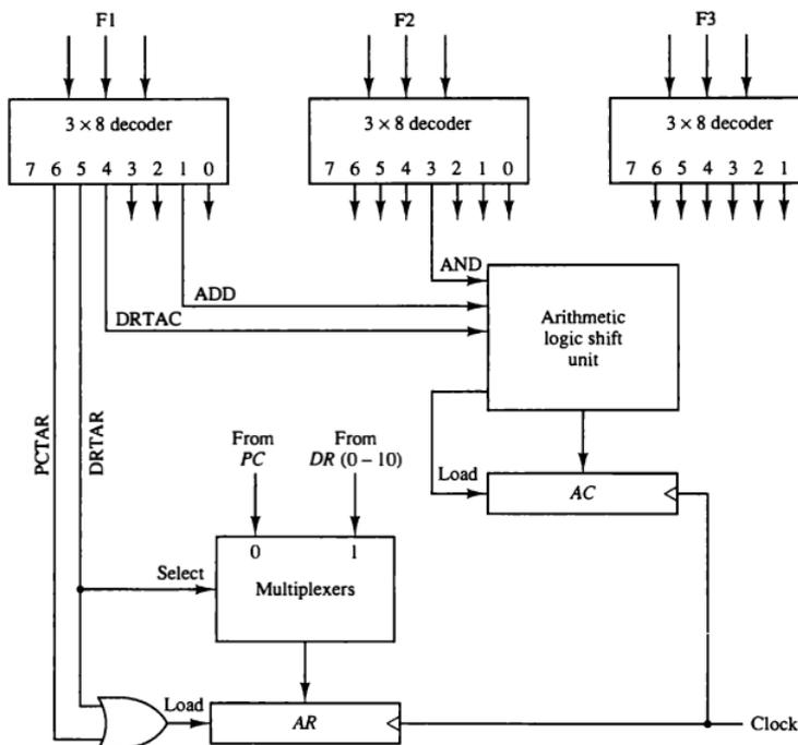
Figure 7-7 Decoding of microoperation fields.
