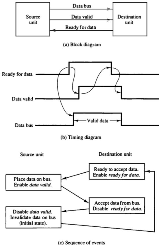
sequence of events in both cases would be identical if we consider the *ready for data* signal as the complement of *data accepted*. In fact, the only difference between the source-initiated and the destination-initiated transfer is in their choice of initial state.
