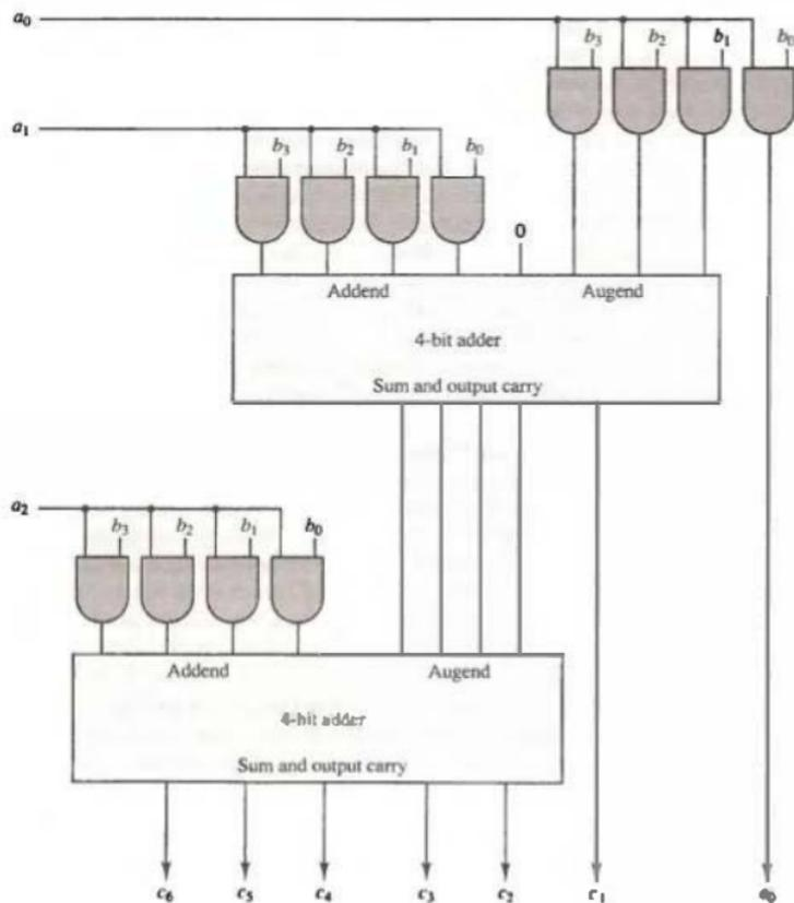
Figure 10.10 4-bit by 3-bit array multiplier.
