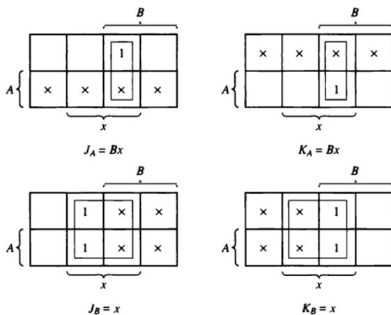
Figure 1-28 Maps for combinational circuit of counter.
