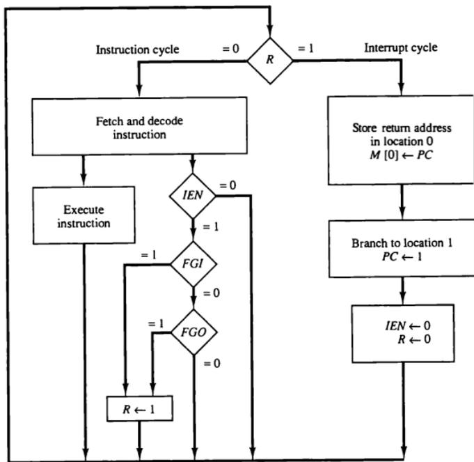
Figure 5-13 Flowchart for interrupt cycle.
