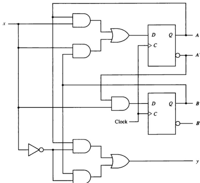
Figure 1-25 Example of a sequential circuit.
