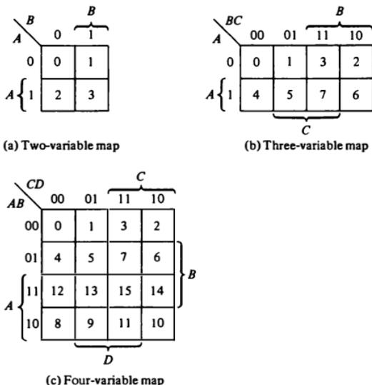
Figure 1-7 Maps for two-, three-, and four-variable functions.
