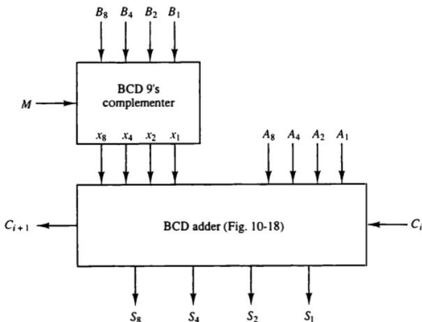
flowcharts can be used for both types of data provided that we interpret the microoperation symbols properly. Decimal numbers in BCD are stored in computer registers in groups of four bits. Each 4-bit group represents a decimal digit and must be taken as a unit when performing decimal microoperations.
