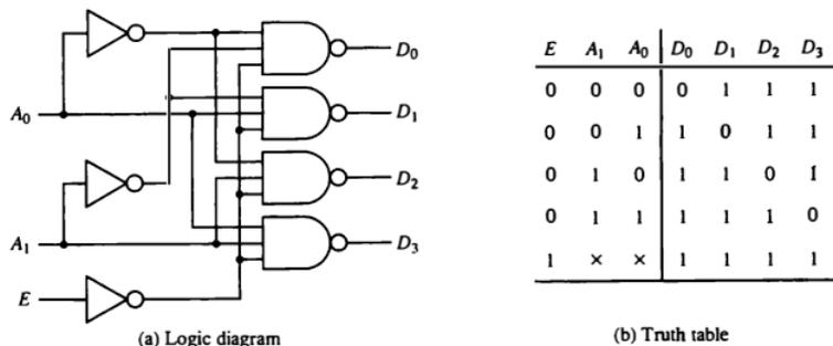
When the circuit is disabled, none of the outputs are selected and all outputs are equal to 1. In general, a decoder may operate with complemented or uncomplemented outputs. The enable input may be activated with a 0 or with a 1 signal level. Some decoders have two or more enable inputs that must satisfy a given logic condition in order to enable the circuit.
