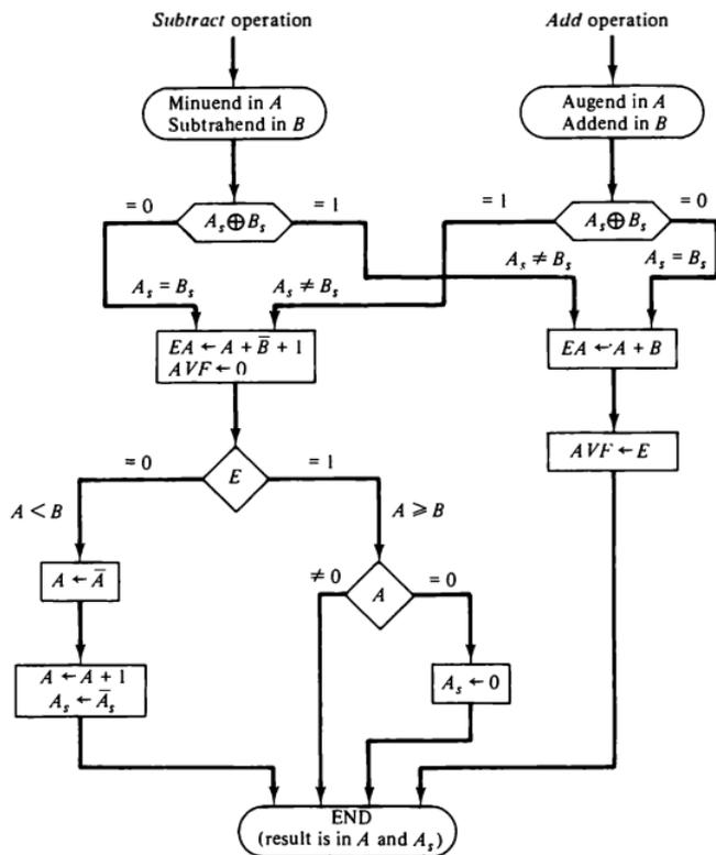
Figure 10-2 Flowchart for add and subtract operations.
