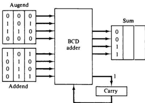
(b) Digit-serial, bit-parallel decimal addition
