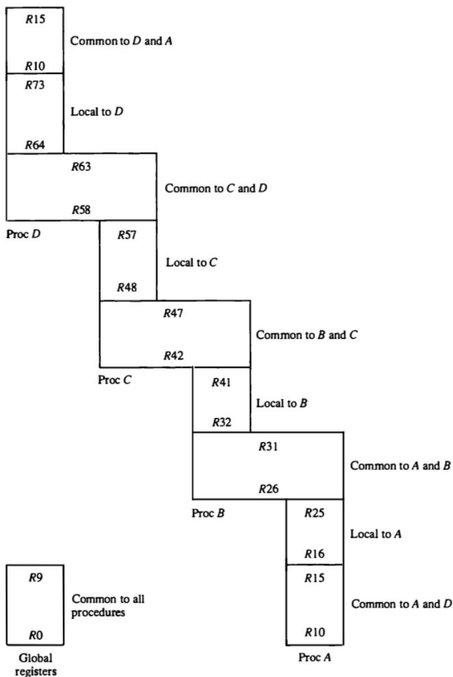
Figure 8-9 Overlapped register windows.
