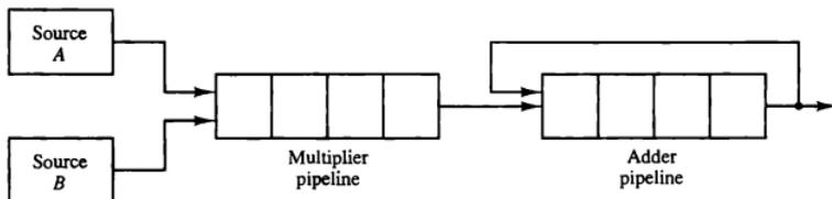
When there are no more product terms to be added, the system inserts four zeros into the multiplier pipeline. The adder pipeline will then have one partial product in each of its four segments, corresponding to the four sums listed in the four rows in the above equation. The four partial sums are then added to form the final sum.
