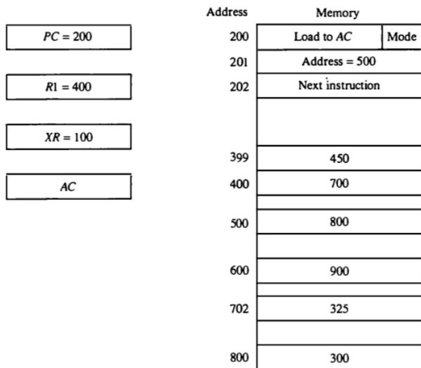
Figure 8-7 Numerical example for addressing modes.
