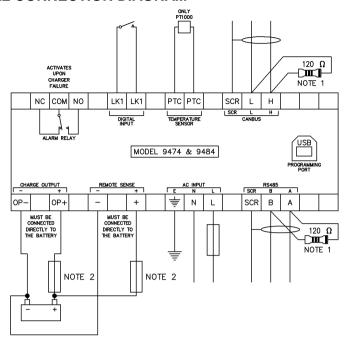
NOTE 1 A 120 OHM TERMINATION RESISTOR MUST BE FITTED IF IT IS THE FIRST OR LAST DEVICE ON THE CANBUS OR RS485 LINK
