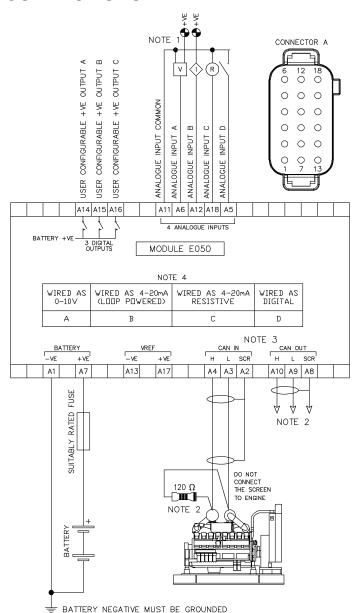
NOTE 1. ANALOGUE INPUT COMMON MUST NOT BE GROUNDED AS IT IS LNIKED INTERNALLY TO TERMINAL A1.
