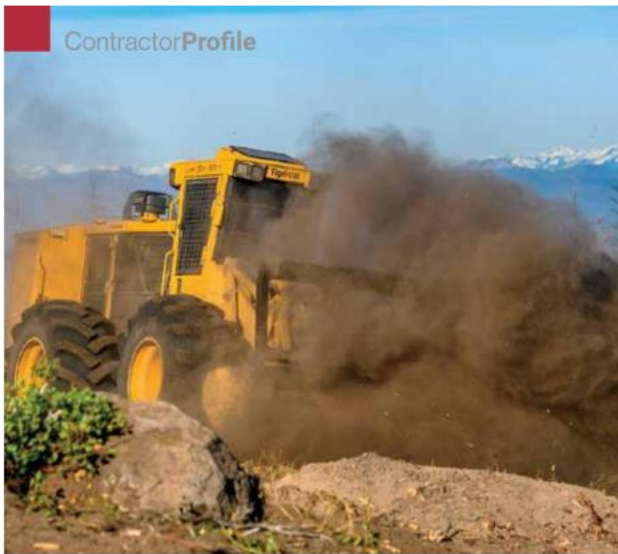
Above and below, company has two of these Tigercat M762G purpose-built mulcher carriers. An optional multi-function hydraulic system and quick-attach boom adapter converts the M726G to a feller buncher for added versatility.
