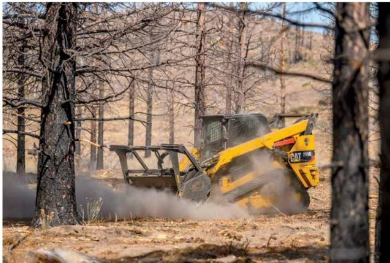
Cat 299D2 skidsteer with Cat mulching attachment. The small skidsteer is effective at mulching but also preventing damage to residual trees.
