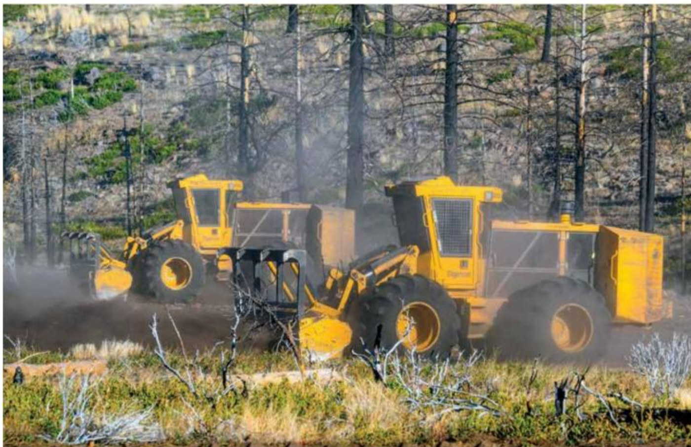
Above and below, company has two of these Tigercat M762G purpose-built mulcher carriers. An optional multi-function hydraulic system and quick-attach boom adapter converts the M726G to a feller buncher for added versatility.
