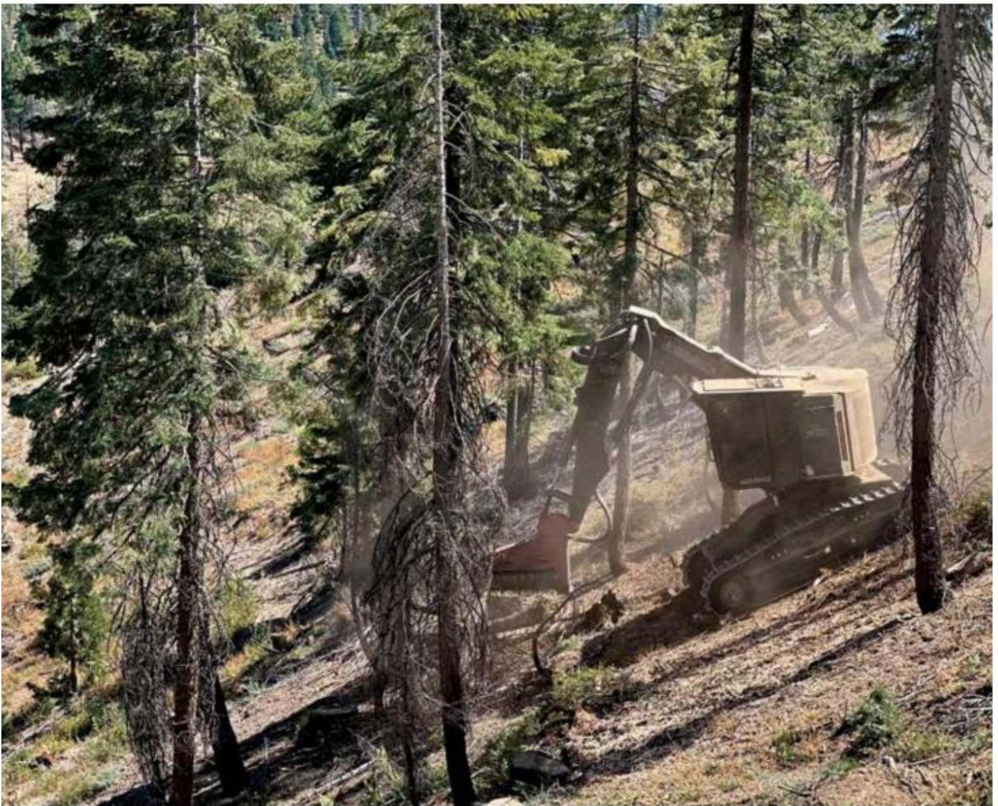
Company's newest machine is this TimberPro 745D with Quadco mulching attachment. Leveling machine is shown helping create a fire break.
