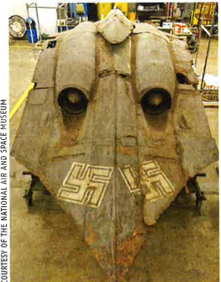
2013 photo (taken just before the start of work and the move to Udvar-Hazy) of the center section, from the rear, showing the "Bat-Wing" tail, as well as the markings added by the Americans.
