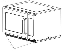
To restall, align the base plate mounting holes, turn the thumbscrews clockwise to tighten.
