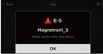
When error code E-1, E-5, E-6 occur and the text description is "Magnetron1\_\*", the "1L" and "4L" symbols get red.
