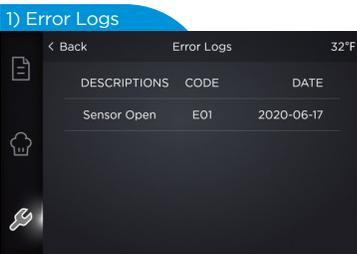
Check the “Error Log” for details of any logged appliance errors and refer to the error codes for more details.
