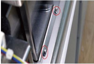
Remove the four M6 nut both side of the cavity.
