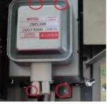
Remove the four M4 screws on both side of magnetron.
