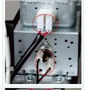
Remove the wire connecting the thermostat and the magnetron.
