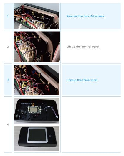
Fitting the control panel
