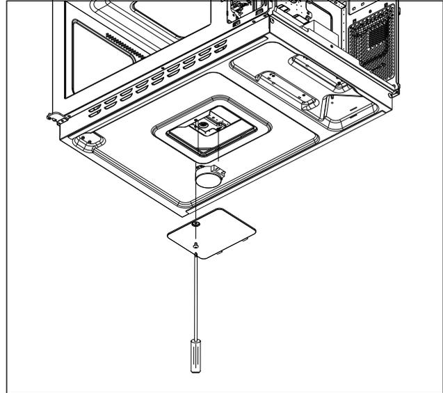
Remove the screws on both side. Take out the whole baseplate assemble.
