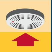
Put the alarm back on the ceiling or wall if it is less than 10 years old.
