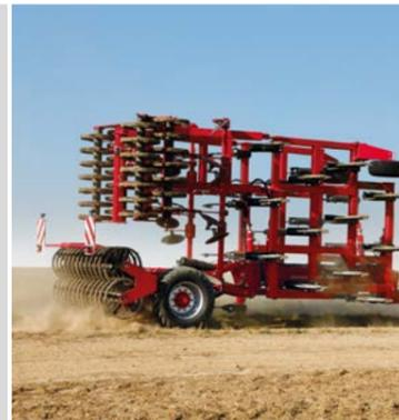
Essieu revolver en position transport
