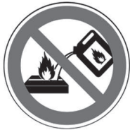
DO NOT FILL WHILE OPERATING
