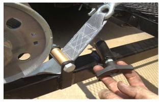
WHEN UNLOADING SCOOTER NEVER LOOSEN WINCH BY MORE THEN 2 FULL TURNS BEFORE YOU RELEASE THE PIN.
