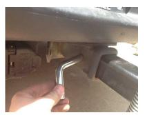
PICK UP (C,D) BY (C) AS SHOWN AND INSERT INTO VEHICLE RECEIVER AS SHOWN THEN INSERT CLEVIS & COTTER PIN TO SECURE.
