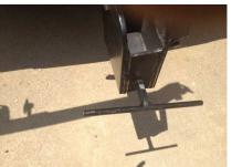
ROTATE T-HANDLE AT BOTTOM (C,D) CLOCKWISE UNTIL UNIT IS FIRM & DOES NOT MOVE OR RATTLE INSIDE THE RECEIVER.
