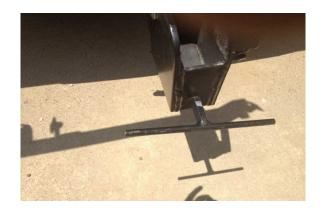
WHEN REMOVING UNIT DO NOT OVER LOOSEN THE T-HANDLE AT BOTTOM OF (D). STOP WHEN THE UNIT BECOMES LOOSE IN THE RECEIVER.
