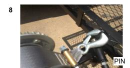
WHEN LEVEL WITH GROUND PULL PIN TO LOCK IN PLACE THEN ATTACH STRAP AND TIGHTEN.
