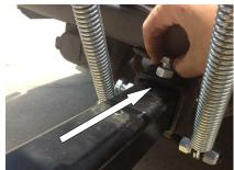
LOOSEN NUTS ON COLLAR NEAR RECEIVER ON (D), MOVE THE COLLAR BACK UNTIL FLUSH WITH RECEIVER, THEN TIGHTEN BOLT 1ST THEN NUT UNDERNEATH 2ND. THIS SETS THE DISTANCE TO MAKE IT EASIER TO LINE UP THE PIN HOLES IN YOUR RECEIVER LATER.
