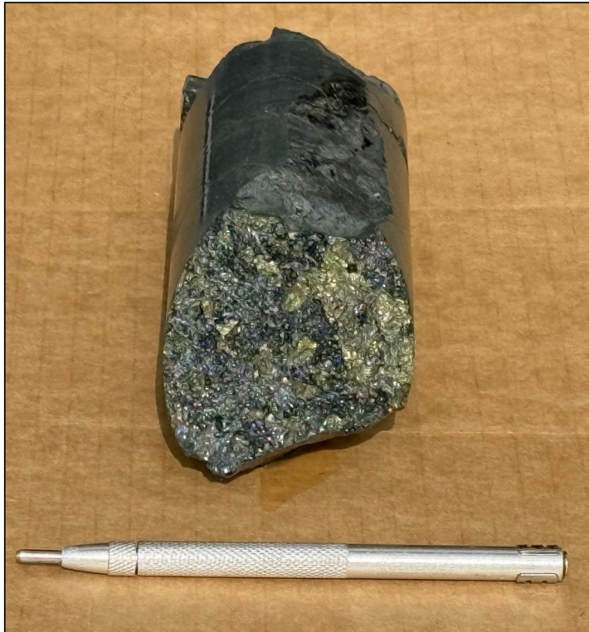
Chalcopyrite, chalcocite and minor pyrite in vuggy quartz vein at 160.7m in SJD001.
