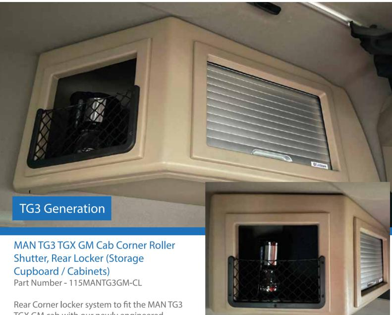
Rear Corner locker system to fit the MAN TG3 TGX GM cab with our newly engineered shutter door system and integrated shelf with cargo net. Microwave and Coffee Maker NOT
