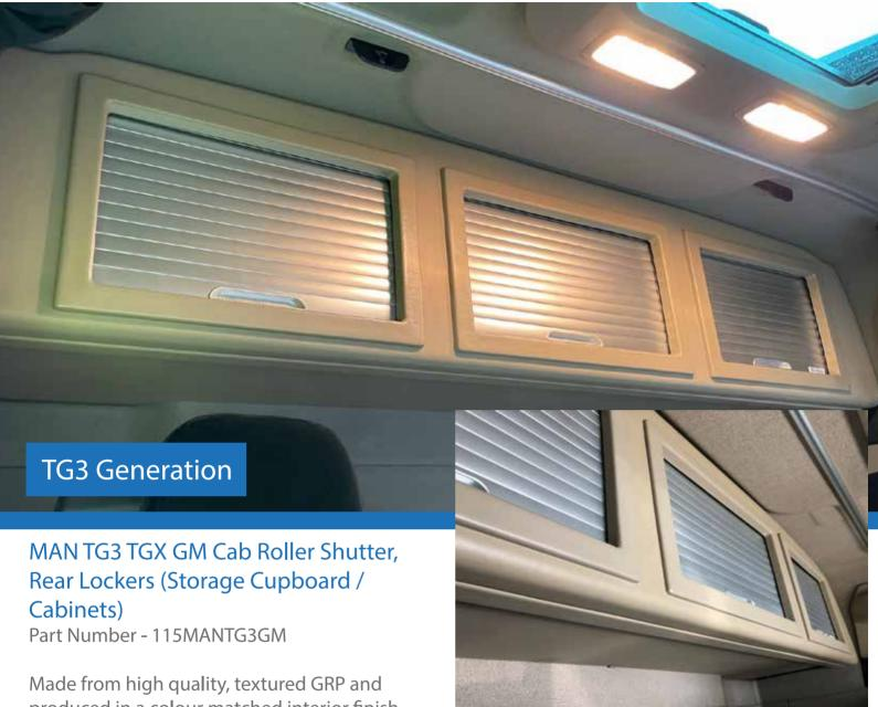
Made from high quality, textured GRP and produced in a colour matched interior finish, combined with a roller shutter door system these lockers have a superb build quality and
