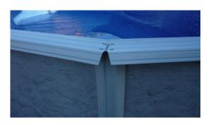
$\Box$  6.3: Insert partially the #10  $\frac{3}{4}$  inch screws on the top. Distribute evenly the space between the top seats to center them between the posts.
