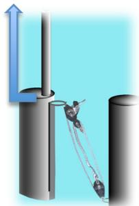
Pull slide up to top of post to allow easy access from patrol boat.
