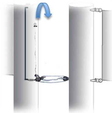
Release tension on rope attached to block and tackle holding fence closed
