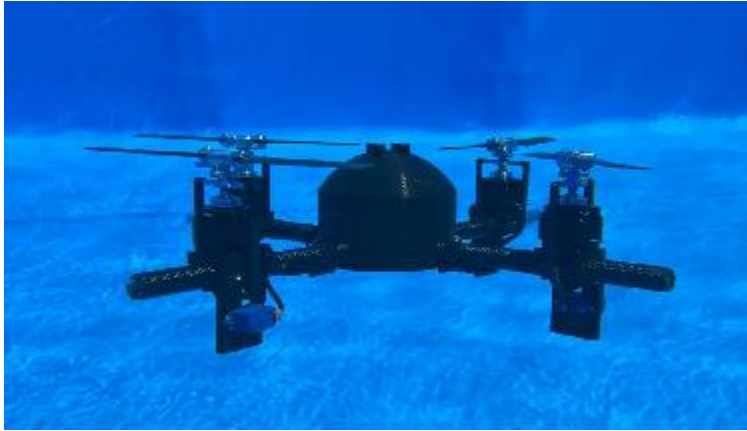
The drone can quickly transition from flying in the air to moving underwater. (Image credit: Andrei Copaci)
