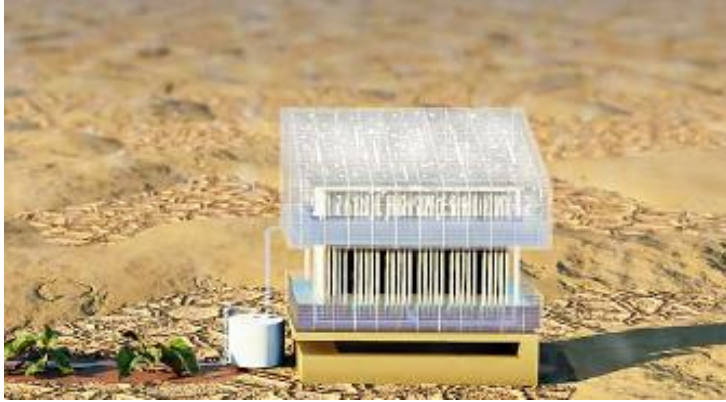
Water out of air A solar-powered water harvester developed by KAUST researchers can extract freshwater at a rate of 2–3 L/m 2 per day during the summer months. (Courtesy: © 2024 KAUST; Heno Hw
