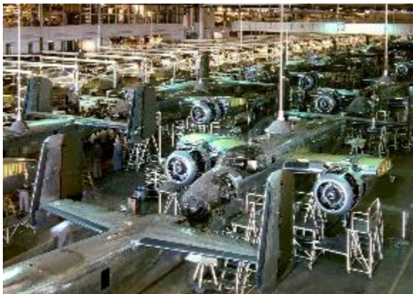
B-25 bombers being assembled in North American Aviation's Inglewood, California factory, 1942 North American Aviation
