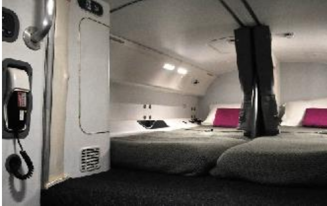
A rest room for pilots, located behind the cockpit of the Boeing 787 Dreamliner. Roslan Rahman/AFP/Getty Images
