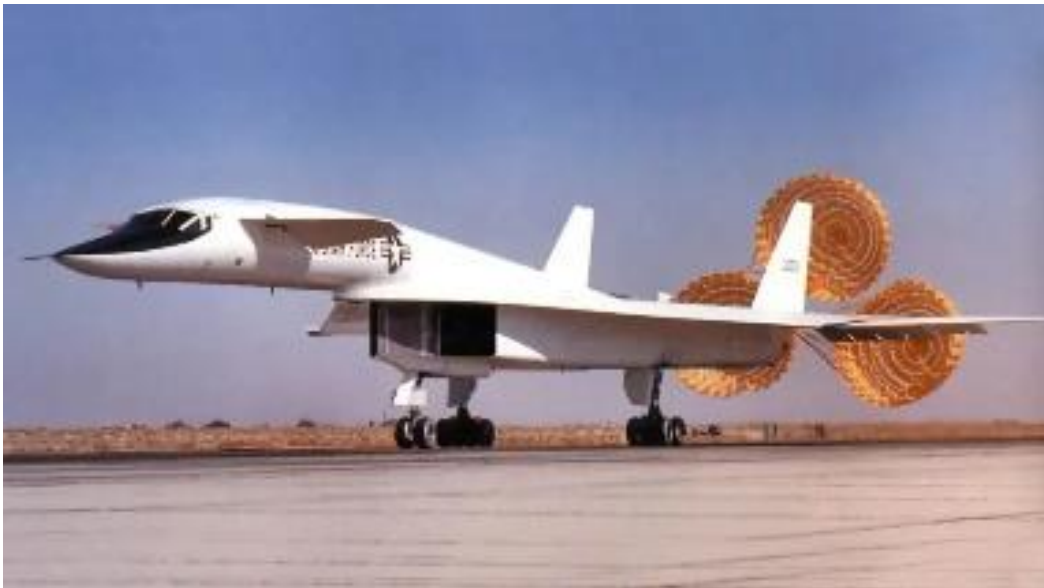
Three drag chutes were needed to slow down the landing roll of the XB-70. (Image credit: Reddit edit The Aviationist)
