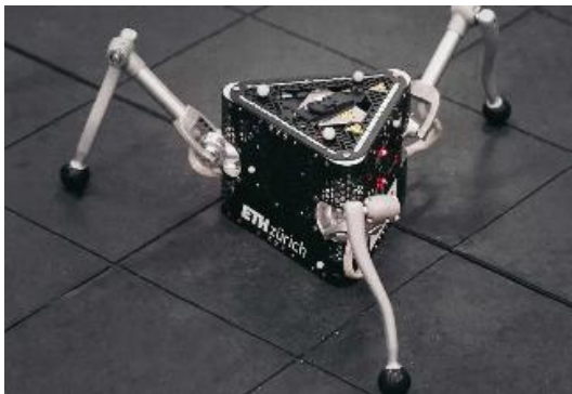
The prototype of the SpaceHopper developed by ETH Zurich students. Dominik Lindegge
