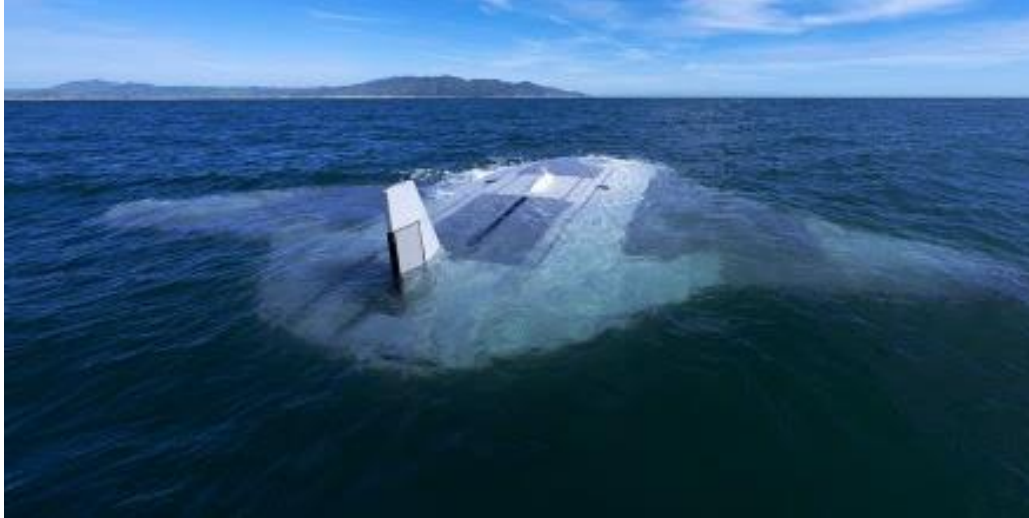
An image of the Manta Ray during in-water testing off the coast of Southern California. This image shows, for the first time, the rear section of the UUV partly submerged (Photos: Northrop Grumman)
