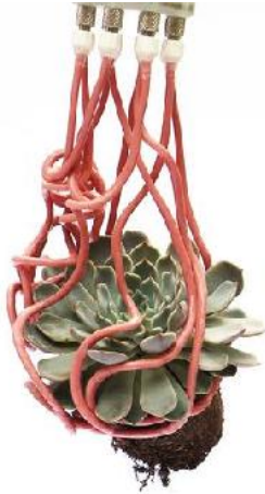
The gripper wrapping around a succulent. (Credit: Harvard Microrobotics Lab/Harvard SEAS)
