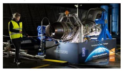
Rolls-Royce says it has run a modified version of a standard jet engine at takeoff power using hydrogen for fuel. The company said it's a key accomplishment in developing future carbon-free designs that can power future aircraft. "This involved overcoming significant engineering challenges as hydrogen burns far hotter and more rapidly than kerosene," Rolls-Royce said. The tests were carried out on a modified Pearl 700 engine.
