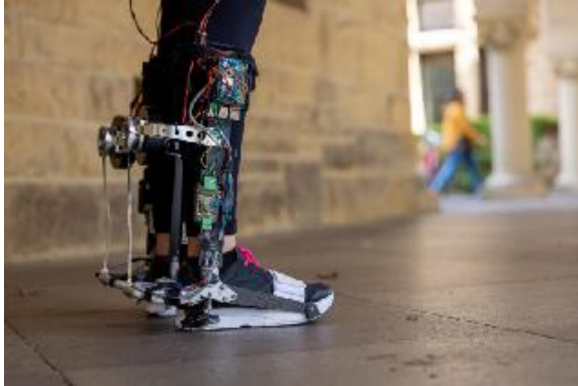
A close-up of the untethered exoskeleton, which monitors movement using inexpensive sensors (Image credit: Kurt Hickman)
