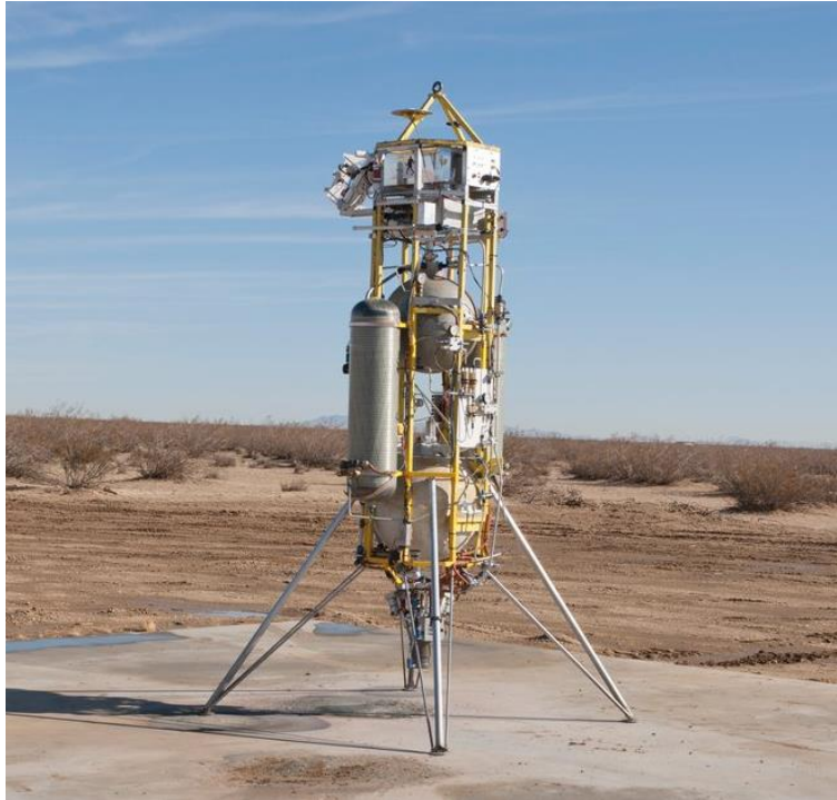
Masten's Xombie VTVL system sits on a launchpad in Mojave, California in December 2014, prepared for a flight test that would help prove lander vision system capabilities for the Mars 2020 Perseverance rover mission.
