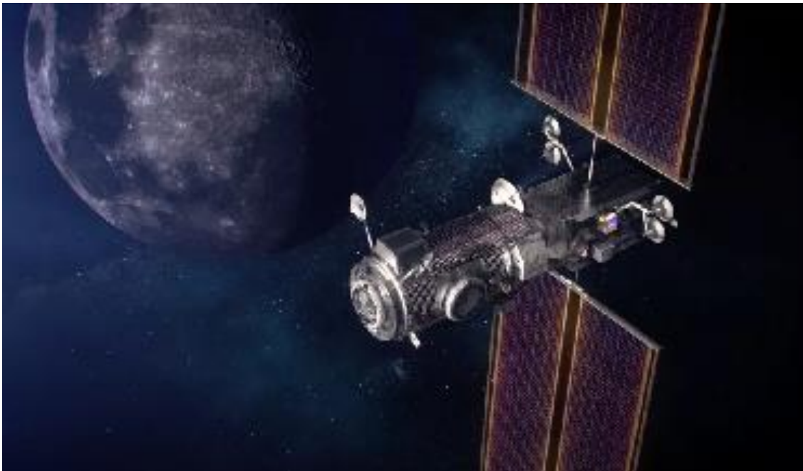
Artist's concept of the Gateway power and propulsion and Habitation and Logistics Outpost (HALO) in orbit around the moon.
